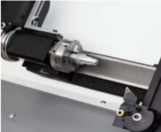
3 Jaw Chuck Holding a machined aluminium part
