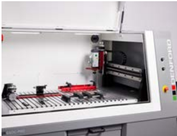
Machine bed with 4 additional Workholding Fixtures
