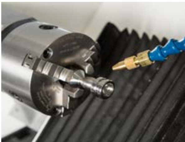
3 Jaw Chuck Holding a machined aluminium part
